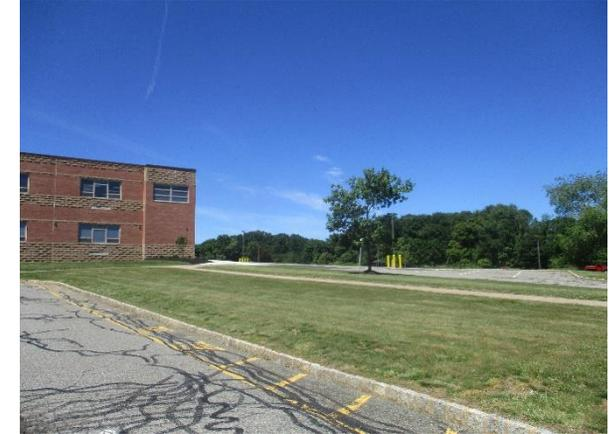
Parking spaces by the north building can be replaced with porous asphalt to infiltrate stormwater. A rain garden south of the building can capture, treat, and infiltrate runoff from the parking lot. A preliminary soil assessment suggests that more soil testing would be required before determining the soil's suitability for green infrastructure.
