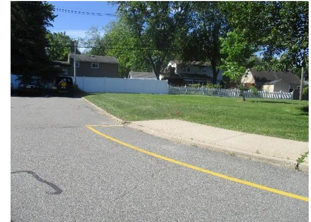
A rain garden adjacent to the parking lot can capture, treat, and infiltrate stormwater runoff. A preliminary soil assessment suggests that the soils have suitable drainage characteristics for green infrastructure.
