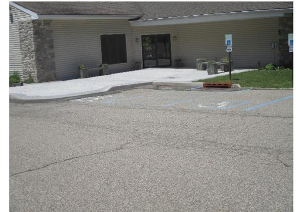
Parking spaces southeast of the building can be replaced with porous asphalt to infiltrate stormwater. A rain garden north of the building can be used to capture, treat, and infiltrate roof runoff. Rainwater can be harvested by installing a cistern at the southwest corner of the building to reuse for watering existing vegetation. A preliminary soil assessment suggests that the soils have suitable drainage characteristics for green infrastructure.
